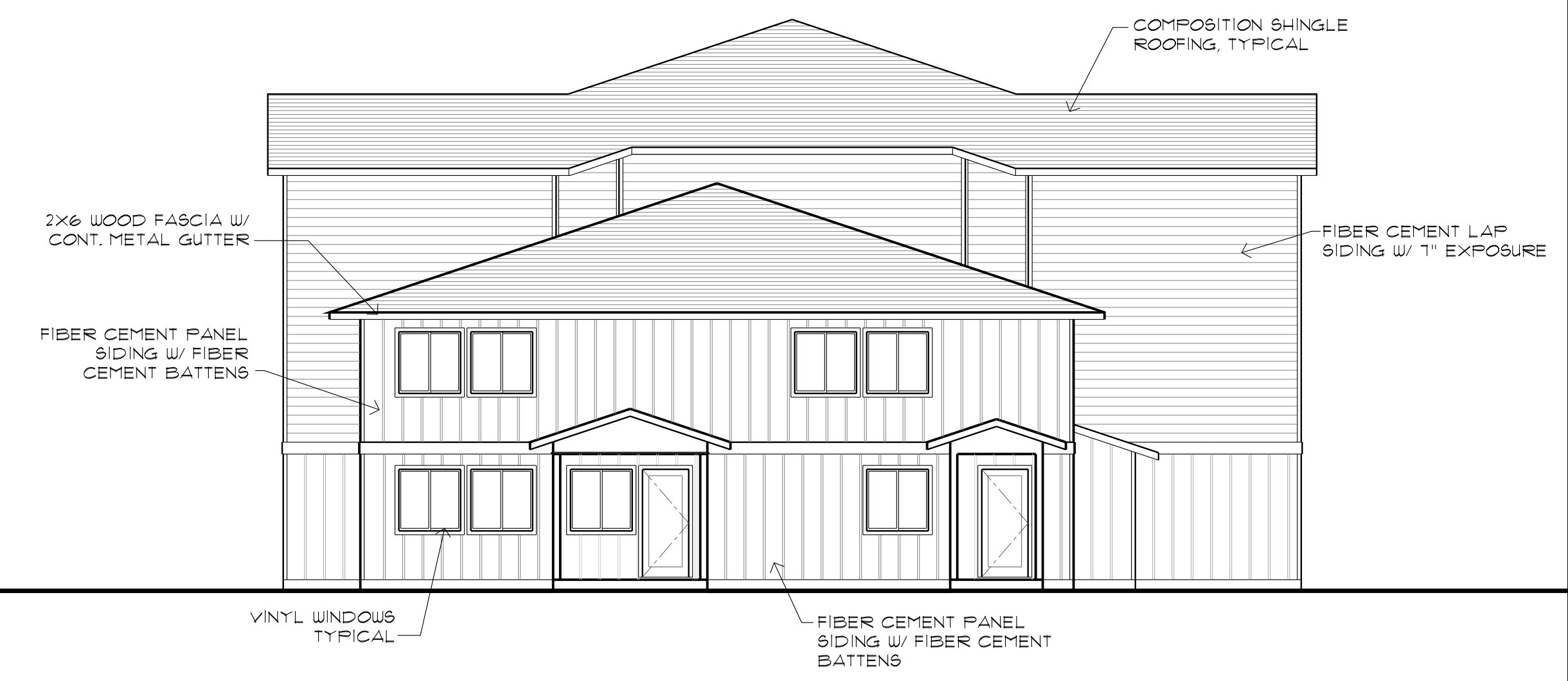
BUILDING 'B' - NORTH ELEVATION 3 Scale: 1/8" = 1'-0" A7.2
