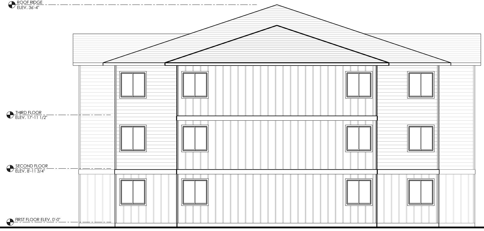
BUILDING 'G' - NORTH ELEVATION 3 Scale: 1/8" = 1'-0" A7.7
