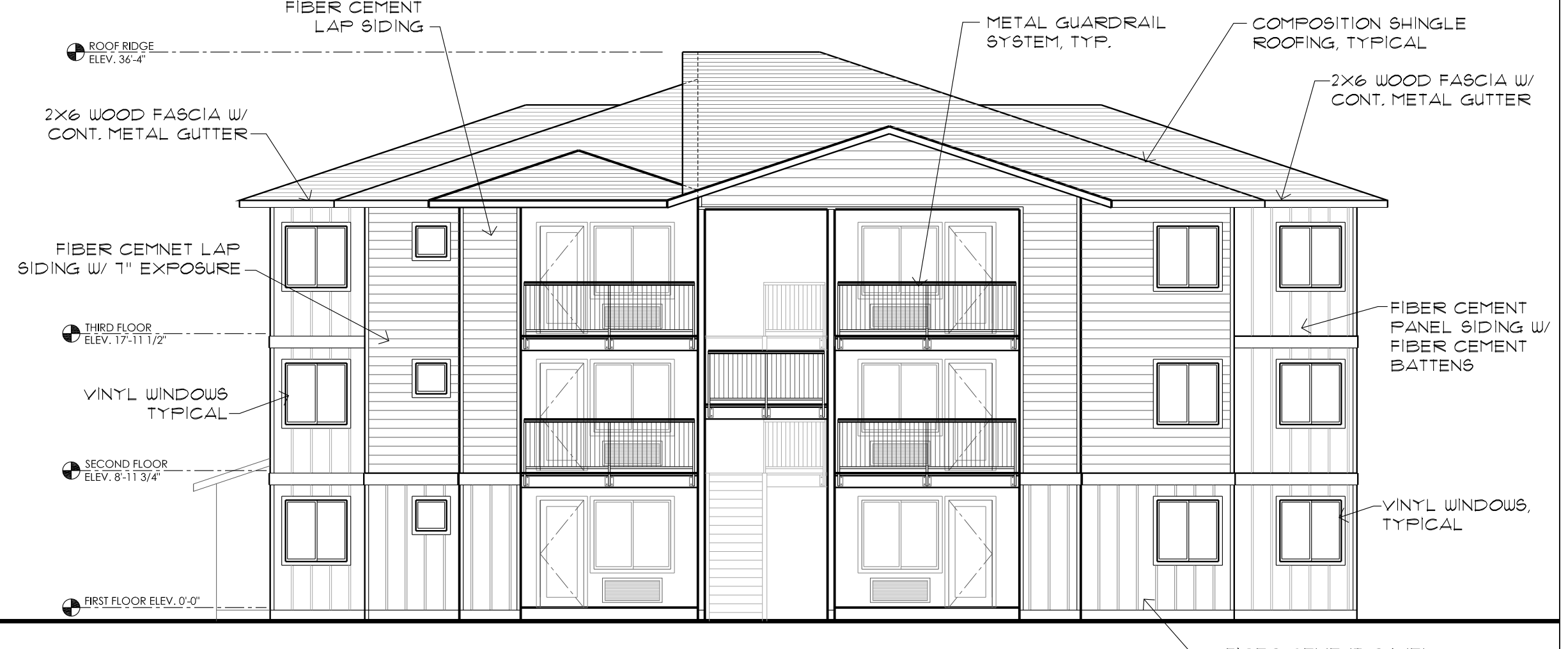
BUILDING 'A' - WEST ELEVATION 4 Scale: 1/8" = 1'-0" A7.1
