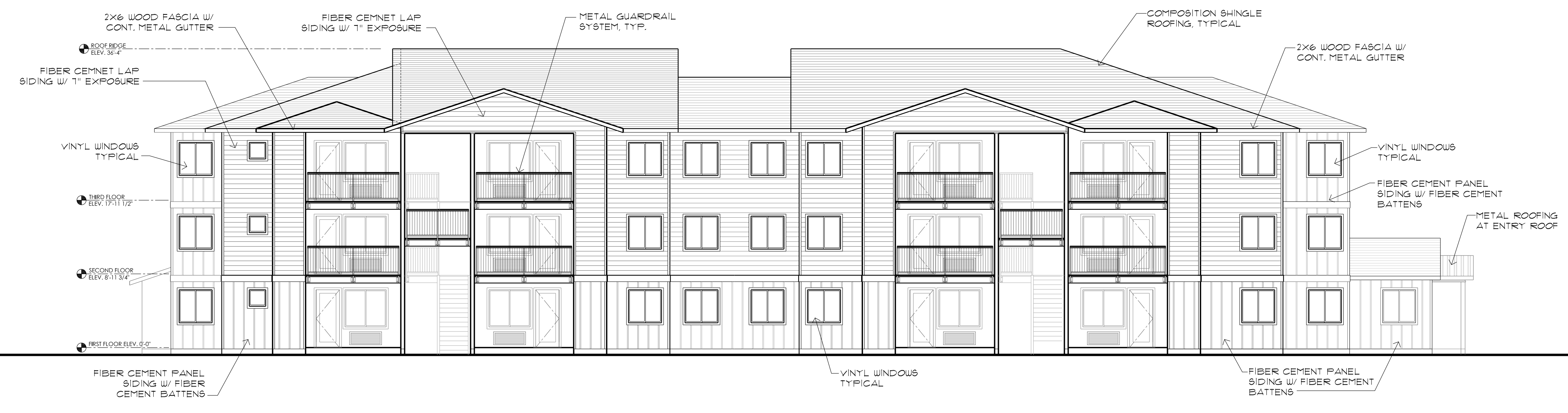
BUILDING 'C' - SOUTH ELEVATION 1 Scale: 1/8" = 1'-0" A7.3
