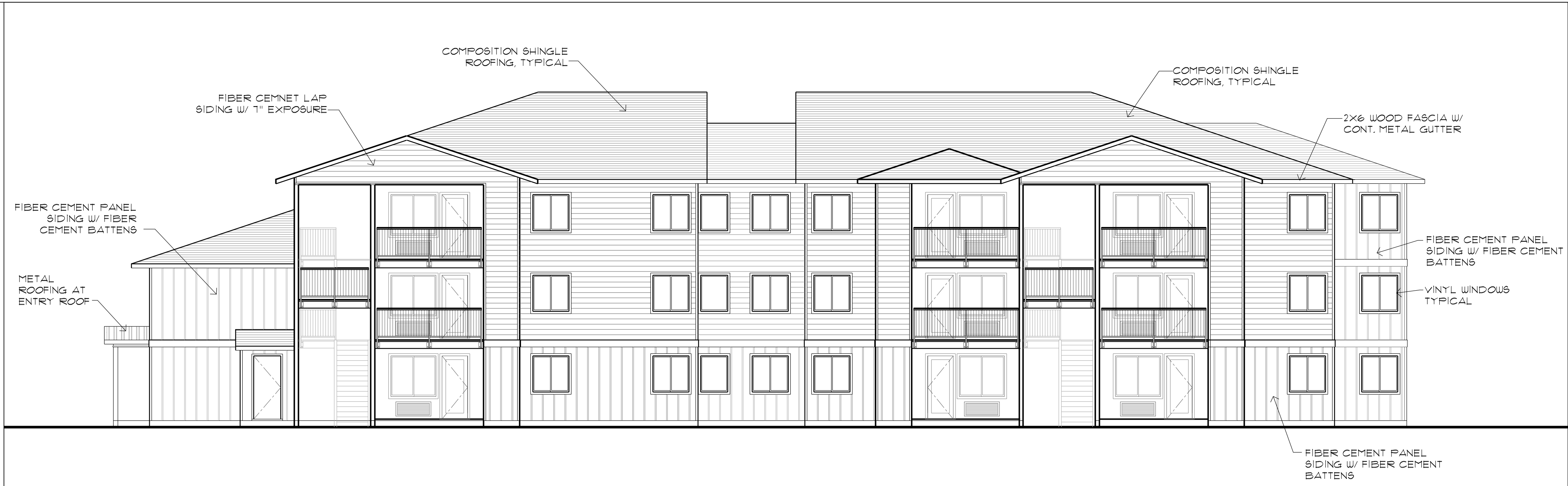
BUILDING 'B' - WEST ELEVATION 4 Scale: 1/8" = 1'-0" A7.2
