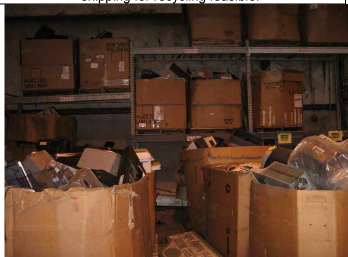
E-waste and CEDs properly stored on pallets and in gayloads
