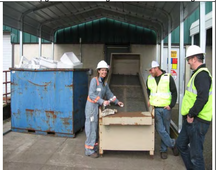
Amanda, Nick and Rick in front of the new styrofoam densifier used to reduce the size of styrofoam to make shipping for recycling feasible.
