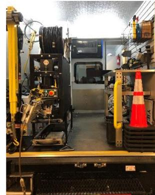
A new van was purchased for the Conveyance System, which is equipped with tools and updated technology used to inspect the sanitary sewer lines, including CCTV cameras which is also pictured.
