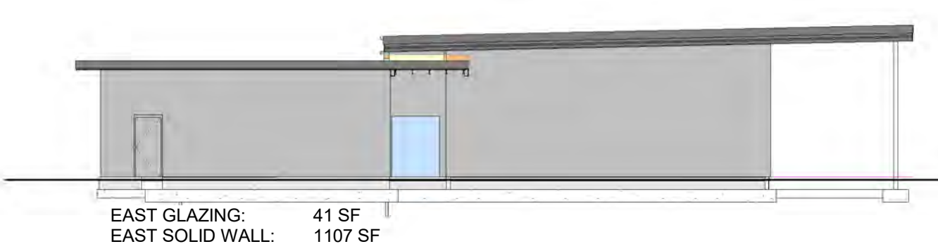
3 GLAZING AREA: EAST ELEVATION G1.10 1/16" = 1'-0"
