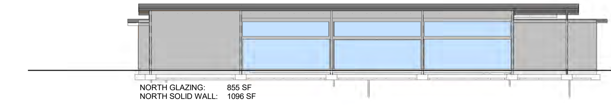
2 GLAZING AREA: NORTH ELEVATION G1.10 1/16" = 1'-0"
