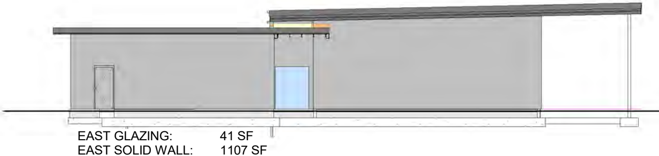
3 GLAZING AREA: EAST ELEVATION G1.10 1/16" = 1'-0"
