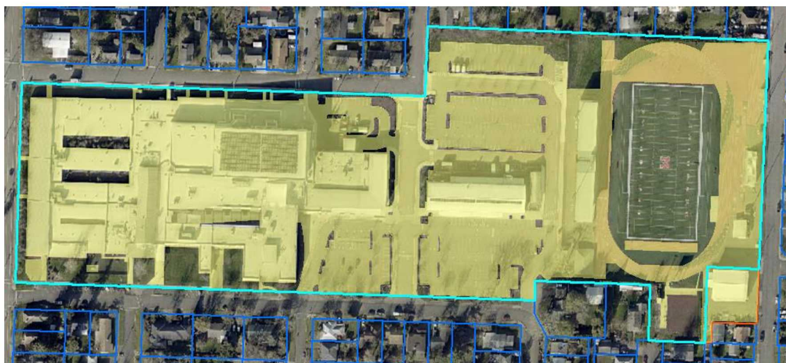
Figure 2. Example of NSFR parcel Impervious Area Digitization (figures not at the same scale)
