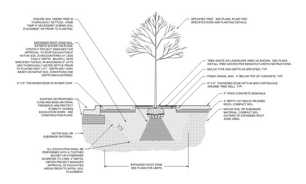
Engineered **Structural Soil** can be compacted as a sturdy base for paving while allowing for easy root growth and overall tree health
