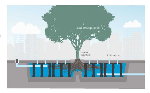
The Silva Cell is a patented modular suspended pavement system that holds unlimited amounts of lightly compacted soil while supporting traffic loads beneath paving. That soil serves two important functions: growing large trees and treating stormwater on-site.
