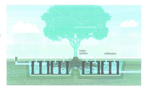
The Silva Cell is a patented modular suspended pavement system that holds unlimited amounts of lightly compacted soil while supporting traffic loads beneath paving. That soil serves two important functions: growing large trees and treating stormwater on-site.
