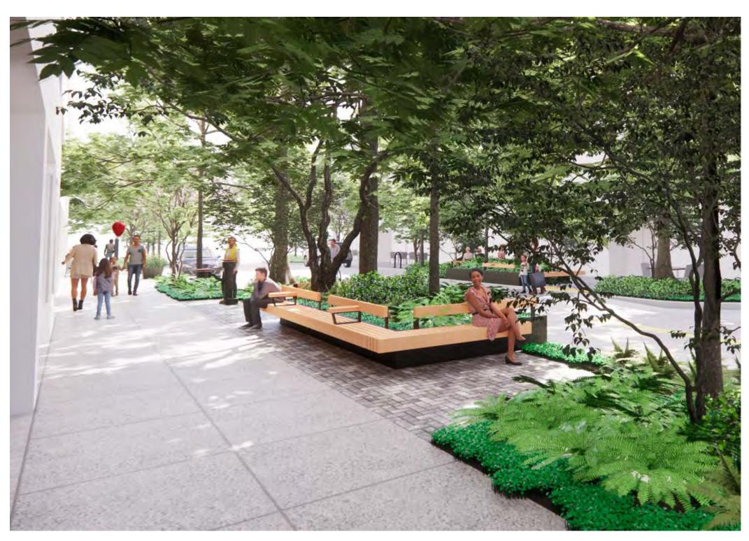
Recommendation: Utilize flush **pavers** of varying sizes/shapes in a tight-fitting layout that maximizes accessibility and minimizes plant growth between pavers
