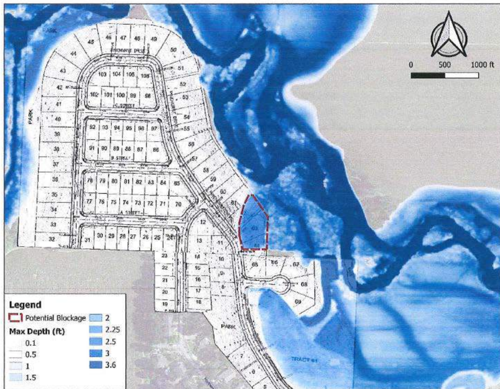
Figure 22: Proposed Condition 100-year Maximum Water Surface Elevation (ft NAVD) Grid Result from RAS Mapper.
